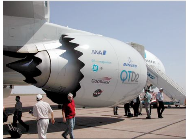
Fig. 16 GE90-155B Turbofan on a Boeing 777 Fitted with SMA-Actuated Chevrons
