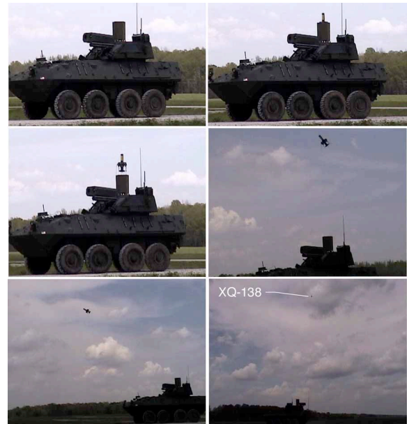
Fig. 10 XQ-138 PBP-Controlled High Performance Convertible UAV Launching, Transitioning and Flying Out from an Armored Vehicle at Redstone Arsenal, AL
