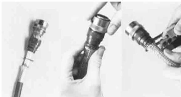
Fig. 3 Raychem Corporation Tinel Lock™ SMA Cable Shielding Termination
